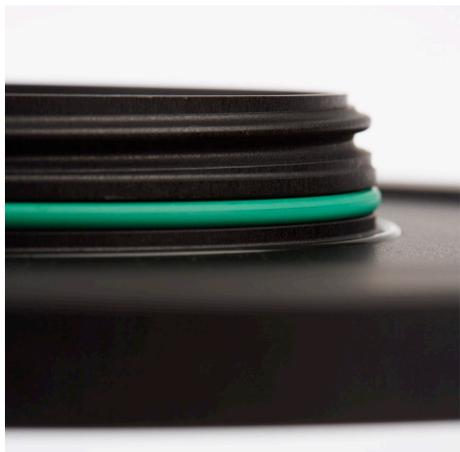
With this specially developed, powerful connection, the bayonet thread pulls the O-ring into the sealing surface with just one turn and positions the port exactly at the stop. The 360° overlap guarantees a secure seal, while a second O-ring provides additional protection against dirt and fine-grained sand.
